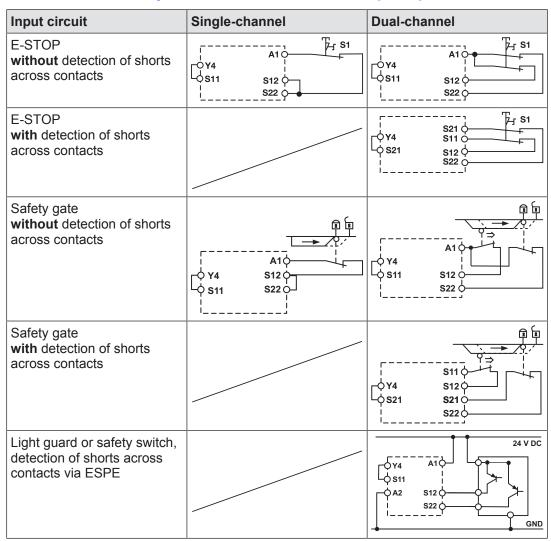
The E-STOP pushbutton and safety gate switch symbolise a trigger element with N/C / N/C combination.
