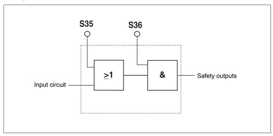
Logic inputs S35 and S36 from the PNOZ e3.1p enable additional PNOZelog or PNOZmulti units to be logically AND/OR connected.
