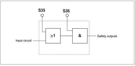
Logic inputs S35 and S36 from the PNOZ e4.1p enable additional PNOZelog or PNOZmulti units to be logically AND/OR connected.
