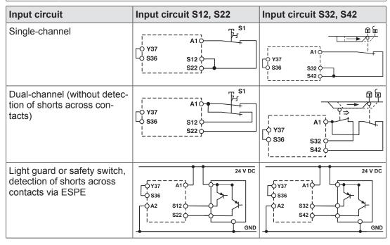
The E-STOP pushbutton and safety gate switch symbolise a trigger element with N/C / N/C combination.
