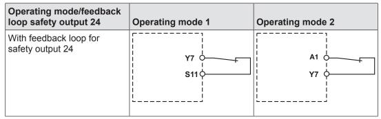
Wiring without a feedback loop is described under "Input circuit".
