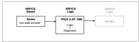
To calculate the safety function you will need the following data for the "sensor" subsystem and the subsystem PNOZ m EF 1MM:
