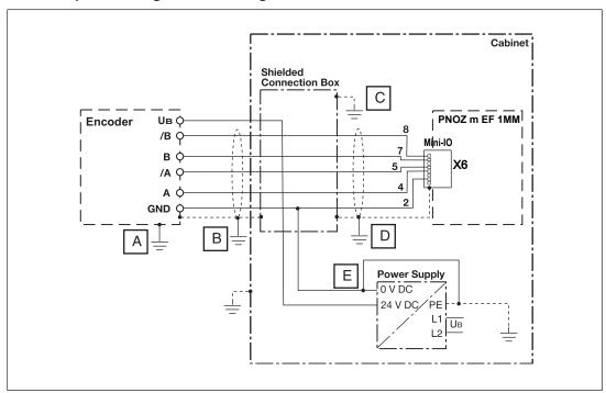
To avoid EMC interference we recommend that the shield on the sensor cables or the housing of the shielded junction box is only connected to earth at a single point:
