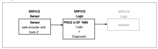
To calculate the safety function you will need the following data for the "sensor" subsystem and the subsystem "PNOZ m EF 1MM":
