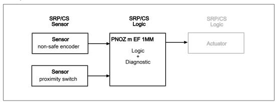
To calculate the safety function you will need the following data for the "sensor" subsystem and the subsystem PNOZ m EF 1MM:
