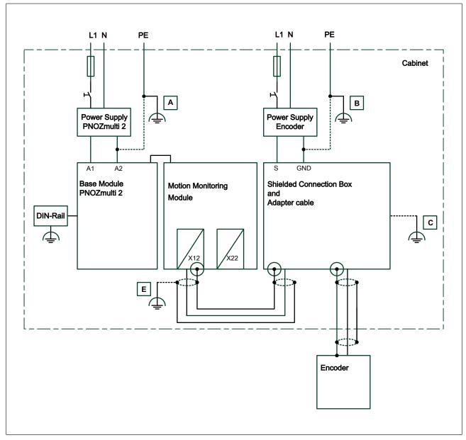
To avoid EMC interference we recommend that the shield on the sensor cable is connected to earth at **C** or **E**. However, depending on the application, it may be helpful to establish the connection to functional earth at another point (in this case **A** or **B**).
