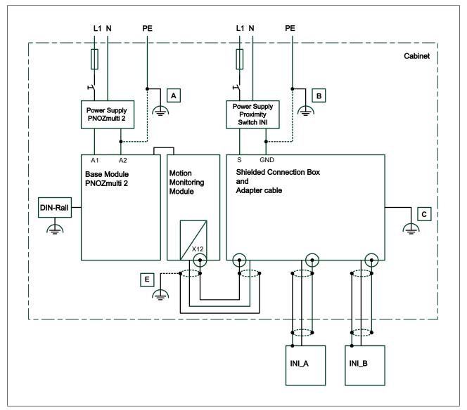
EMC-compliant wiring for connecting 2 proximity switches
