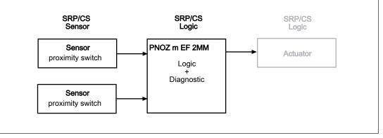
The supply voltage of the proximity switches must be monitored as a measure against systemic failure.
