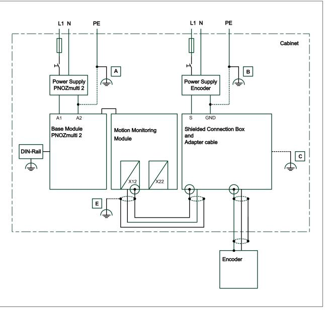
EMC-compliant wiring for connecting an encoder
