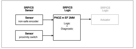
To calculate the safety function you will need the following data for the "sensor" subsystem and the subsystem PNOZ m EF 2MM:
