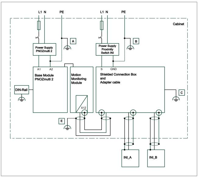
EMC-compliant wiring for connecting 2 proximity switches
