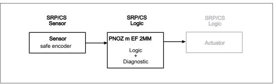
To calculate the safety function you will need the following data for the "sensor" subsystem and the subsystem "PNOZ m EF 2MM":
