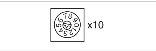
On the middle rotary switch x10, use a small screwdriver to set the tens digit for the address ("3" in the example).
