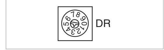
On the upper rotary switch DR, use a small screwdriver to set the transmission rate (in the example, "3" corresponds to 50 kBit/s).
