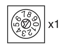
On the lower rotary switch x1, set the ones digit for the address ("6" in the example). Station address 36 is set in the diagrams as an example.
