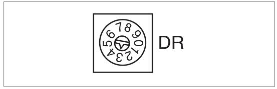
▶ On the upper rotary switch DR, use a small screwdriver to set the transmission rate (in the example, "3" corresponds to 50 kBit/s).
