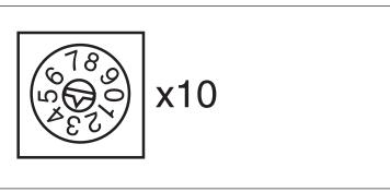
▶ On the upper rotary switch x10, use a small screwdriver to set the tens digit for the address ("3" in the example).
