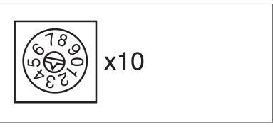
▶ On the middle rotary switch x10, use a small screwdriver to set the tens digit for the address ("3" in the example).
