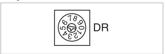
▶ On the upper rotary switch DR, use a small screwdriver to set the transmission rate (in the example, "3" corresponds to 50 kBit/s).
