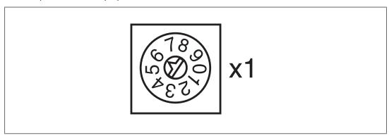
▶ On the lower rotary switch x1, set the ones digit for the address ("6" in the example). Station address 36 is set in the diagrams as an example.
