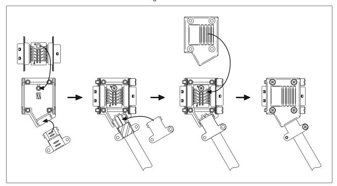
The cable clip is suitable for cables with a diameter of 3 mm - 12 mm
