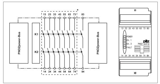
\*Safe separation from non-marked area, except for safety contact 83-84, in accordance with EN 60947-1, 6 kV, basic insulation between all safety contacts.
