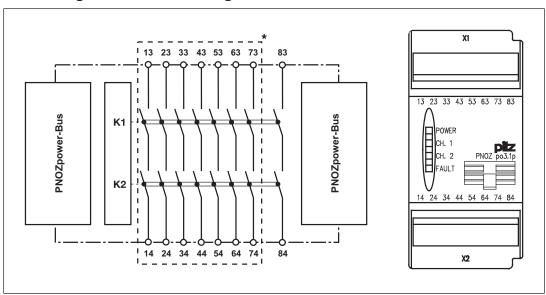
\*Safe separation from non-marked area, except for safety contact 83-84, in accordance with EN 60947-1, 6 kV, basic insulation between all safety contacts.
