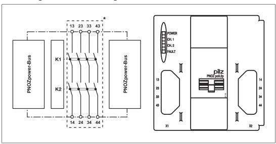
\*Safe separation from non-marked area in accordance with EN 60947-1, 6 kV, basic insulation between all safety contacts.
