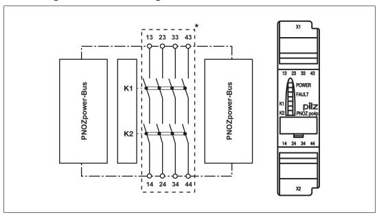
\*Safe separation from non-marked area in accordance with EN 60947-1, 6 kV, basic insulation between all safety contacts.
