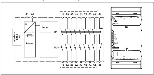
\*Safe separation from non-marked area in accordance with EN 60947-1, 6 kV, basic insulation between all safety contacts.
