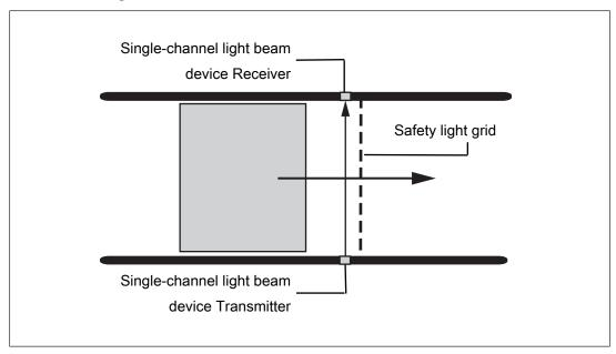
The transmitter emits a light beam, which is reflected by the receiver. If an object interrupts the light beam, the receiver detects this and muting is activated.
