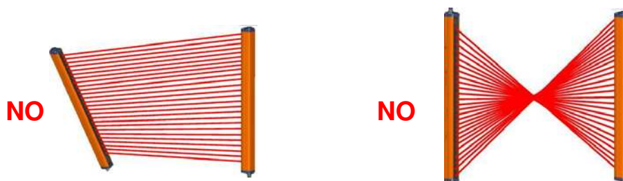
Fig. 14 – Light curtain alignment
