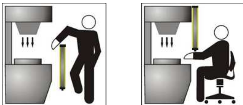
Fig. 5 – Device positioned incorrectly
