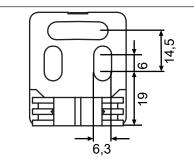
Bore holes in the installation surface (two M6 screw boreholes per flexible bracket) for mounting the flexible brackets for the transmitter and receiver.
