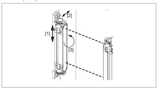
Fig.: Transmitter/receiver modification directions during orientation
