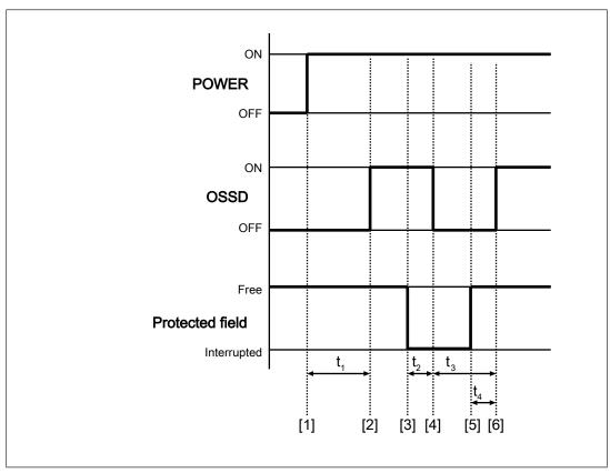
Fig.: Automatic start and restart timing diagram
