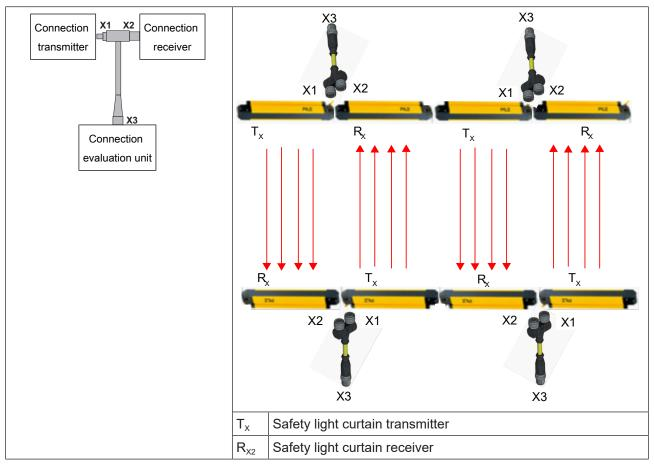
▶ Example: save on cable when making connections in the control cabinet
