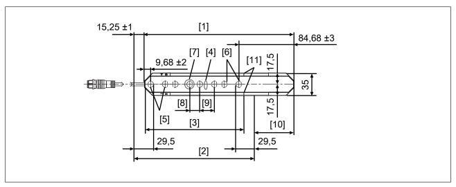
Fig.: Front view of the safety light curtain transmitter, protected field height 150 mm with connection cable
