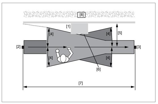
Fig.: Interference with the function of the safety light curtain due to reflective surfaces – top view
