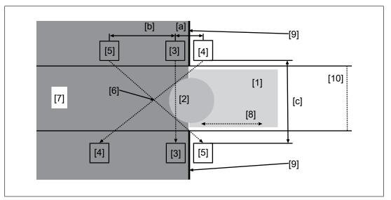
Fig.: Arrangement of the muting sensors with cross muting
