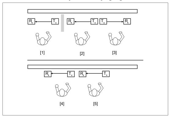
Fig.: Using several adjacent safety light curtains
