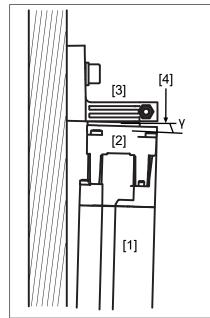
Uneven installation surfaces can be compensated for with the standard installation kit to a limited extent only.
