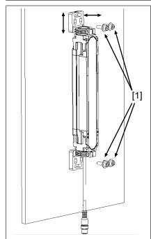
Fix the transmitter and receiver and their flexible brackets in place on the installation surface.
