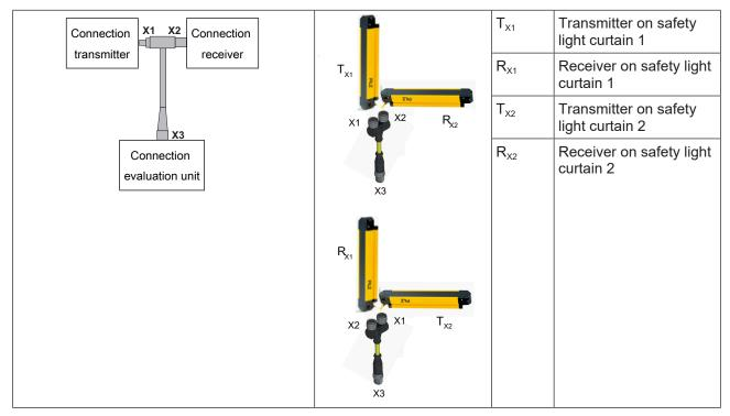
Example: install parallel-aligned safety light curtains next to each another
