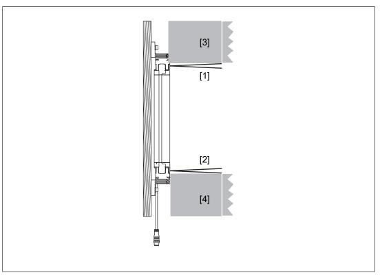
Fig.: Placement of the dead zones in vertical safety light curtain installation
