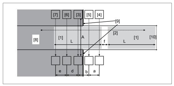
Fig.: Arrangement of the muting sensors with T-muting
