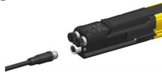
Fig. 4 Connection in the foot area of the safety light curtain
