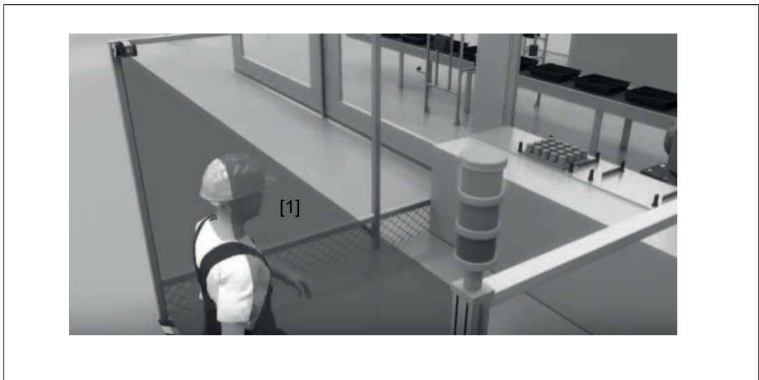
Fig.: Application example PSENscan safety laser scanner - vertical configuration
