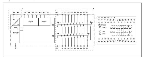
\*Insulation against the non-marked area and between the relay contacts: Basic insulation (overvoltage category III), protective separation (overvoltage category II)
