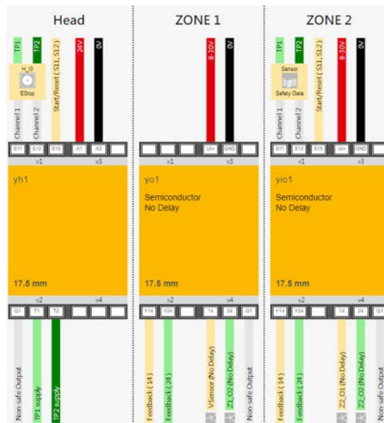
Figure 15 - Connection diagram myPNOZ with semiconductor outputs
