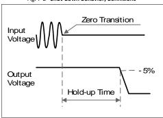
Note: At no load, the hold-up time can be up to several seconds. The green DC-OK LED is on during this time.
