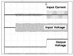
Input: 230Vac Output: 24V, 10A Ambient: 25°C
