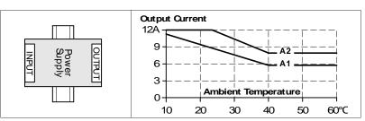
Fig. 22-8 Mounting Orientation E (Horizontal ccw)
