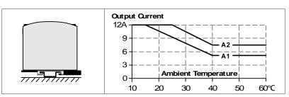
Fig. 22-7 Mounting Orientation D (Horizontal cw)
