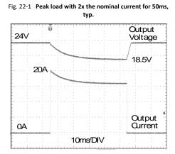
20A Peak load (resistive) for 50ms Output voltage dips from 24V to 18.5V.
