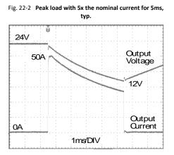
50A Peak load (resistive) for 5ms Output voltage dips from 24V to 12V.
