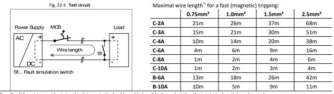
\*) Don't forget to consider twice the distance to the load (or cable length) when calculating the total wire length (+ and – wire).
