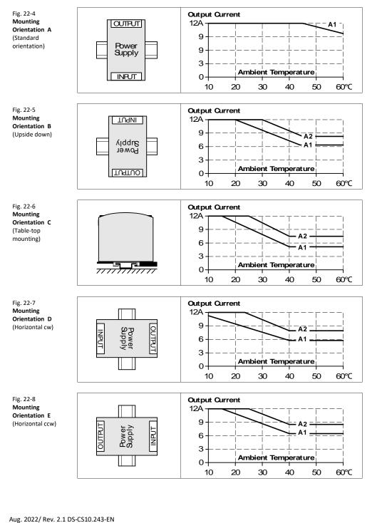
All parameters are specified at 24V, 10A, 120Vac, 60Hz, 25°C ambient and after a 5 minutes run-in time unless otherwise noted.
