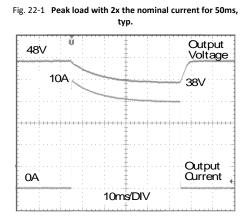
10A Peak load (resistive) for 50ms Output voltage dips from 48V to 38V.
