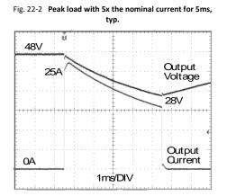
25A Peak load (resistive) for 5ms Output voltage dips from 48V to 28V.
