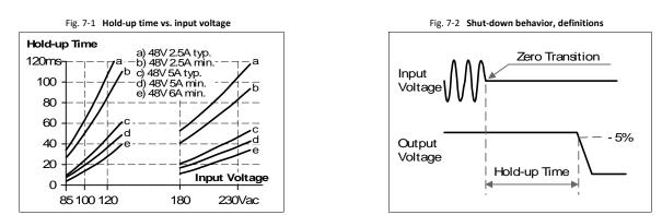
Note: At no load, the hold-up time can be up to several seconds. The green DC-OK LED is on during this time.
