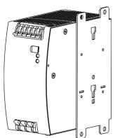
Side mounting without DIN-rail brackets
