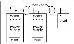
Fig. 22-7 Using distribution terminals
