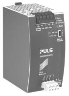
This buffer unit is a supplementary device for DC 48V power supplies. It delivers power to bridge typical mains failures or extends the hold-up time after turn-off of the AC power. In times when the power supply provides sufficient voltages, the buffer unit stores energy in integrated electrolytic capacitors. In case of mains voltage fault, this energy is released again in a regulated process. One buffer module can deliver 20A additional current.
