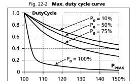
$$DutyCycle = \frac{T_{peak}}{T_{peak} + T_0}$$
