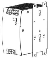
Side mounting without DIN-rail brackets
