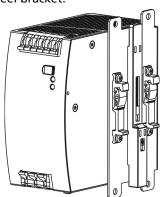
Side mounting with DIN-rail brackets
