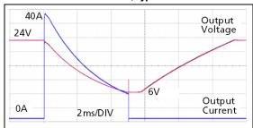
Peak load 40A (resistive load) for 5ms Output voltage dips from 24V to 6V.
