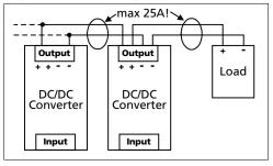
Fig. 11-2 Using distribution terminals
