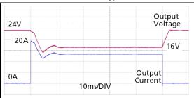
Peak load 20A (resistive load) for 50ms Output voltage dips from 24V to 16V.
