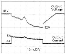
Fig. 23-3 7.5A peak current for 12ms, typ. (3x the nominal current)
