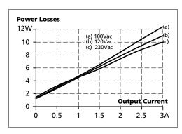
Fig. 9-4 Losses vs. input voltage at 48V, 2.5A, typ.
