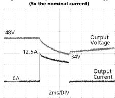
Please note: The DC-OK relay triggers when the voltage dips more than 10% for longer than 1ms.
