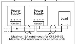
Fig. 12-2 Using distribution terminals
