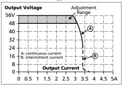
Fig. 6-2 **Dynamic output current capability, typ.**
