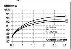
Fig. 9-3 **Efficiency vs. input voltage at 48V, 2.5A, typ.**
