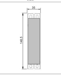
Fig. 22-5 **Hole pattern for wall mounting**
