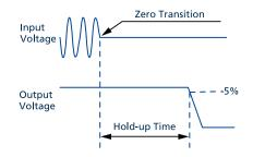
Fig. 7-2: Shut-down behaviour, definitions
