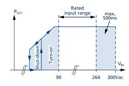
Fig. 3-1: Input voltage range
