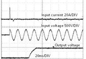
Fig. 5-3: Typical turn-on behavior at 230Vac and 25°C ambient
