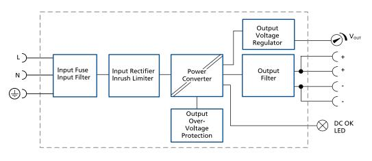
Fig. 11-1: Functional diagram
