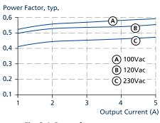
Fig. 3-4: Power factor vs. output load at 12V output voltage
