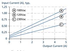
Fig. 3-3: Input current vs. output load at 12V output voltage
