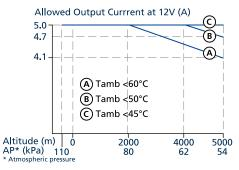
Fig. 15-2: Output power vs. altitude
