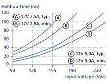
Fig. 7-1: Hold-up time vs. input voltage
