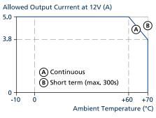
Fig. 15-1: Output power vs. ambient temp.
