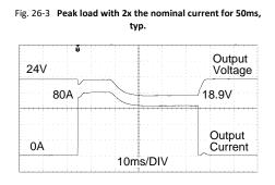
80A Peak load (resistive) for 50ms Output voltage dips from 24V to 18.9V.
