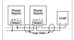
Fig. 15-2 Using distribution terminals
