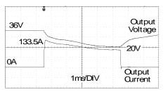
133.5A Peak load (resistive) for 5ms Output voltage dips from 36V to 20V.
