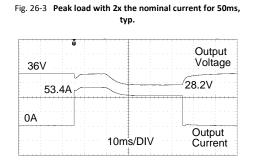
53.4A Peak load (resistive) for 50ms Output voltage dips from 36V to 28.2V.
