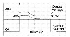
40A Peak load (resistive) for 50ms Output voltage dips from 48V to 37.9V.
