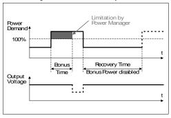
The BonusPower is available as soon as power comes on and after the end of an output short circuit or output overload.
