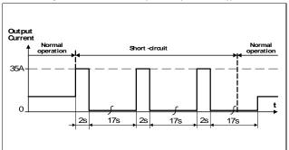
Fig. 6-4 Dynamic overcurrent capability, typ.
