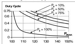
$$DutyCycle = \frac{T_{peak}}{T_{peak} + T_0}$$
