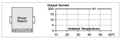
Fig. 26-7 Mounting Orientation B (Upside down)
