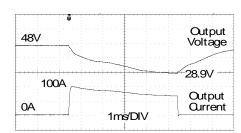
100A Peak load (resistive) for 5ms Output voltage dips from 48V to 28.9V.
