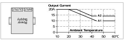
Fig. 26-8 Mounting Orientation C (Table-top mounting)
