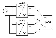
Energize all units at the same time to avoid the overload Hiccup<sup>PLUS</sup> mode. It also might be necessary to cycle the input power (turn-off for at least five seconds), if the output was in Hiccup<sup>PLUS</sup> mode due to overload or short circuits and the required output current is higher than the current of one unit.
