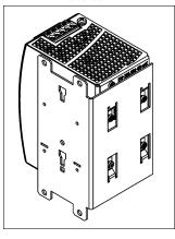
Fig. 25-4 Side mounting with DIN rail brackets
