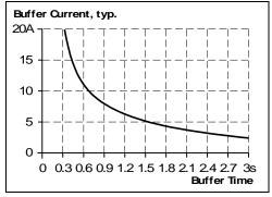
Fig. 6-2 Buffer time for small buffer currents, typ.
