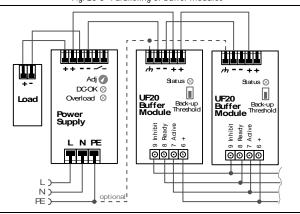
Fig. 26-4 Decoupling of buffered branches
