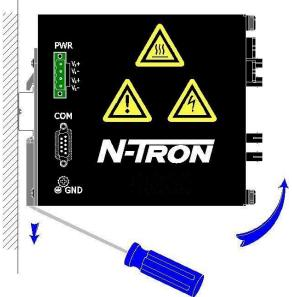
To remove the unit from the 35mm din-rail, place a flat head screwdriver into the release clip at the bottom of the unit, and push down on the clip until it disengages from the bottom of the unit from the din-rail. Lift the om bott of the unit up at an approximate 45° upward angle to completely remove the unit.
