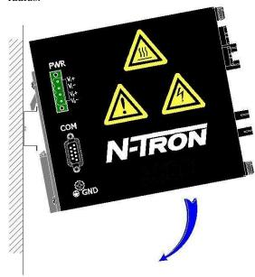
To mount the unit to the 35mm din-rail, place top edge of the bracket on the back of the unit against the din-rail at a  $45^{\circ}$  upward angle. Lower the bottom of the unit until it snaps into place.
