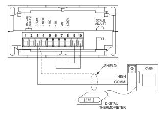
A biscuit baker has temperature controllers on his ovens that have a dial for setting the temperature of his ovens. He would like to have a digital display of his temperature for ease of monitoring. He has determined, by talking to the temperature controller manufacturer, there is a 0 to 10 VDC voltage available from the controller, that represents a temperature of approximately 0 to 600°F.
