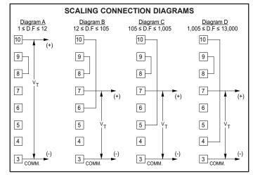
**EXAMPLE 2:** A tachometer generator delivers 210 VDC at maximum machine speed which is to be indicated as 575 FPM on an Apollo Voltmeter.
