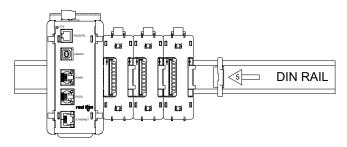
Figure 3 - Attach Termination Plug\*
