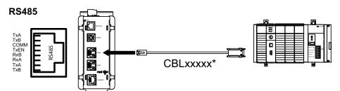
**WARNING:** Do **NOT** use a standard DH-485 cable to connect this port to Allen Bradley equipment.
