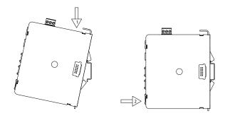
Figure 1 - Attach CSMSTR Master To DIN Rail
