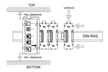
Figure 2 - Attach Slave Bases To DIN Rail
