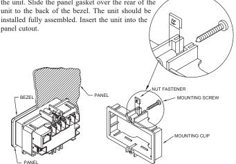
While holding the unit in place, push the panel latch over the rear of the unit so that the tabs of the panel latch engage in the slots on the case. The panel latch should be engaged in the farthest forward slot possible. To achieve a proper seal, tighten the latch screws evenly until the unit is snug in the panel (Torque to approx. 28 to 36 in-oz [0.202 to 0.26 N-m]). Do not over-tighten the screws.
