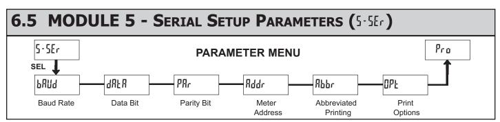
The Serial Setup Parameters are only active when one of the optional serial communication/programming cards is installed in the meter. Refer to the CUB5COM bulletin for details on CUB5 RS232 or RS485 serial communications.
