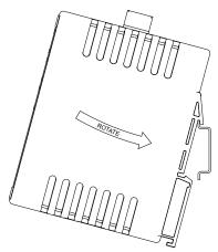
The unit shall be installed inside a UL Listed Industrial Control Panel or similar type of enclosure. A minimum 3.2 mm distance shall be maintained between the hazardous live parts of the equipment and accessible parts of the fire/electrical enclosure.
