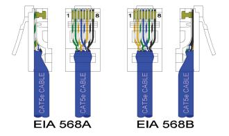
be utilized. If a user does not follow one of these standards then the performance and maximum cable distance will be reduced significantly, and may prevent the switch from establishing a link.
