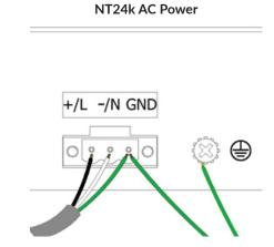
For the DIN rail models, see the illustration below for grounding:
