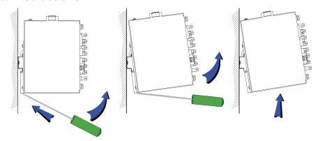
Remove the switch from standard 35mm DIN rail as shown in the diagram above.
