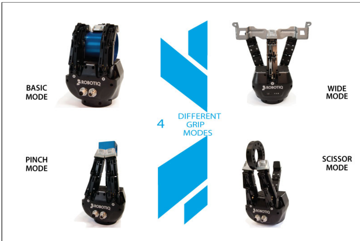
Figure 1.3 : The four Operation Modes of the Adaptive Gripper.
