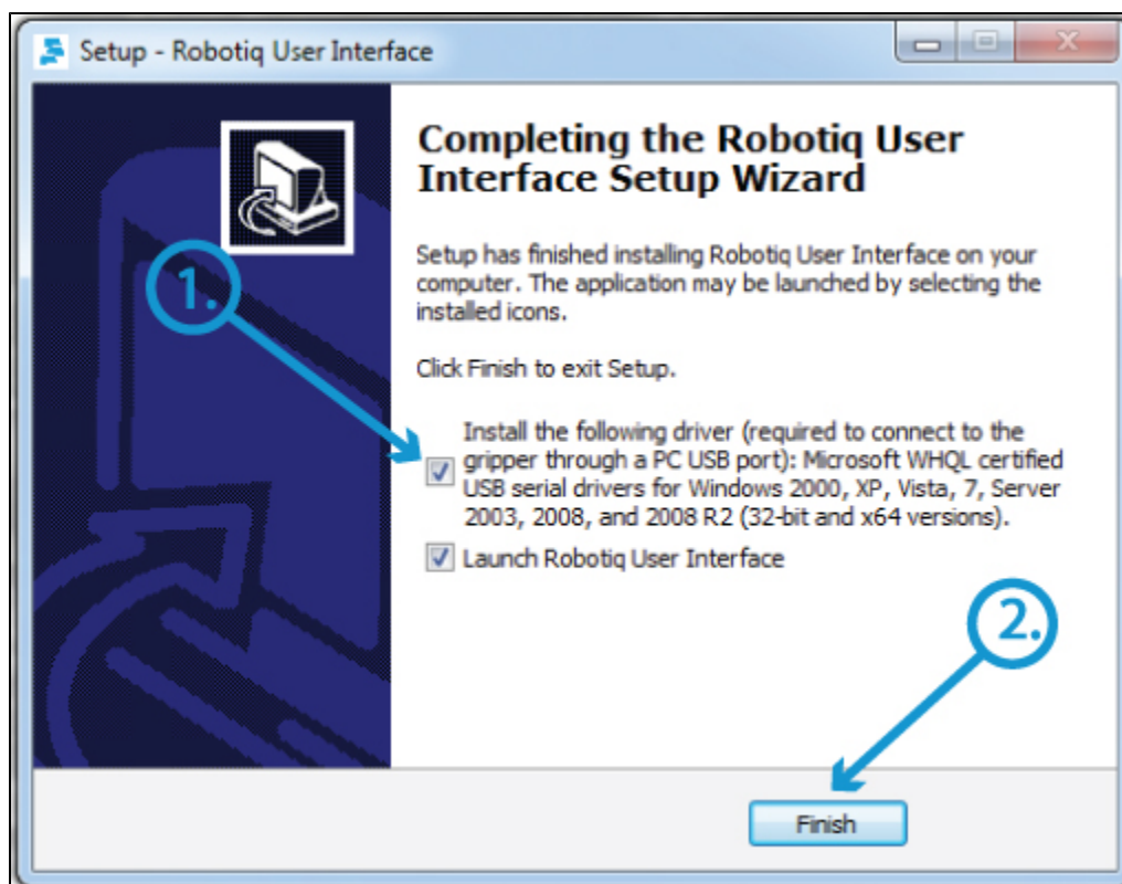
Figure 5.2.1 : Completing the installation of Robotiq User Interface
