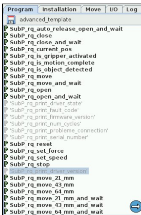
Fig. 1-1: Older program's subprograms to suppress or rename to use with URcaps package.
