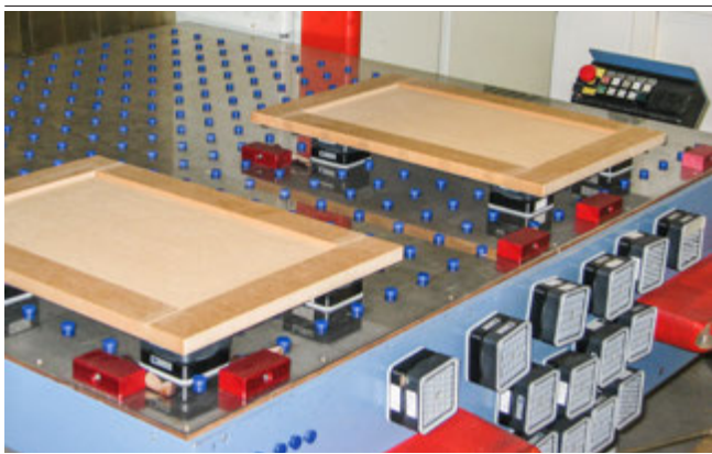
Innospann Steel-Plate with Mono-Base and suction cups
