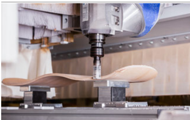
Aluminum Vacuum Block VCBL-A-K2 for clamping solid wood
