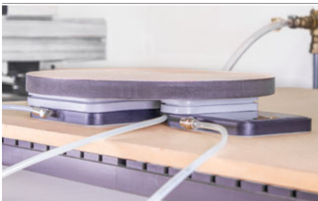
Vacuum Blocks VCBL-G-K1 for clamping MDF workpieces
