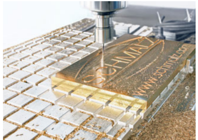
Vacuum clamping system Matrix-Plate MPL for engraving a brass sign
