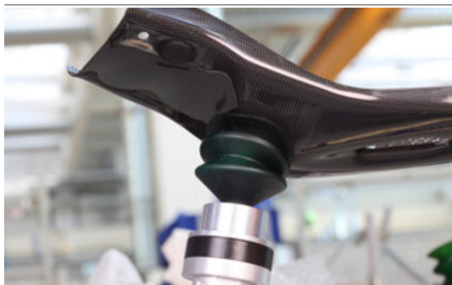
Uni-Base UB and Reference suction cup RSC for clamping carbon fiber-reinforced plastic parts
