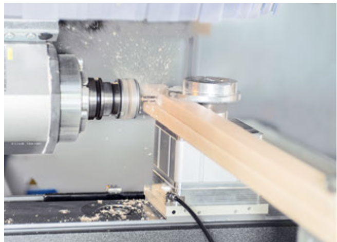
Mechanical clamp VCMC-K1 for processing narrow frame parts
