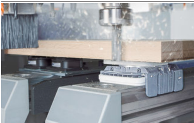
Vacuum Block VCBL-K1 for clamping solid wood
