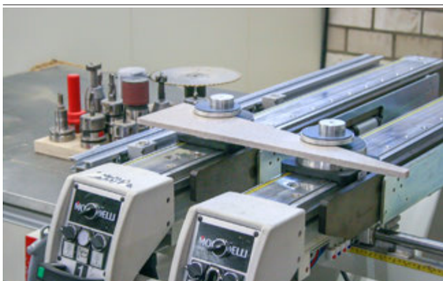
Mechanical Clamps VCMC-S4 for clamping wooden parts
