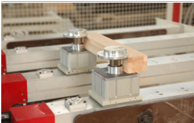
Mechanical Clamps VCMC-K2 for clamping frame parts
