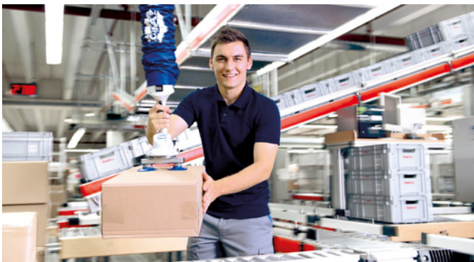
Vacuum tube lifter Jumbo for light loads
