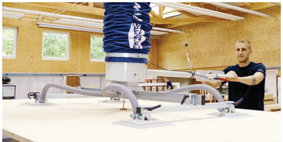
Vacuum tube lifter for heavy wooden boards
