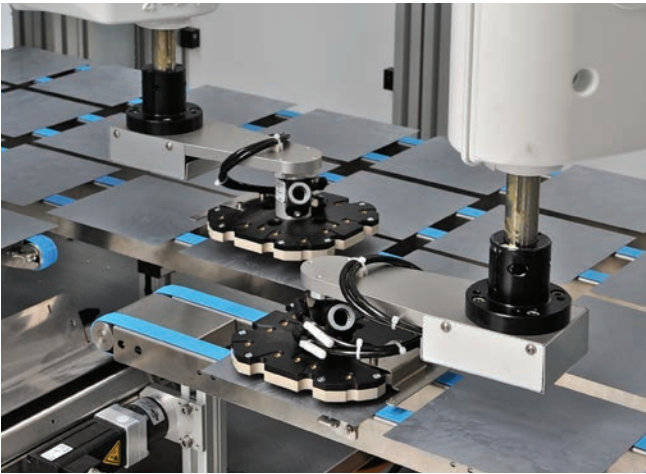
Wafer gripper SWGm handling solar wafers in a solar panel manufacturing process
