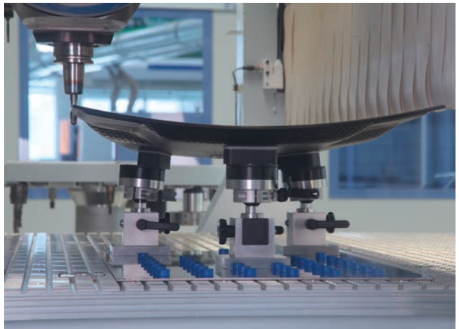
Vacuum block BHF for positioning and fixing a hardened composite textile workpiece during edge machining
