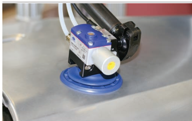
Decentralized vacuum generation with ejector SEAC RP with blow off system right on suction cup
