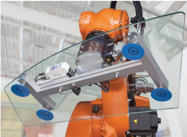
Vacuum suction cups SAB on a spider with central vacuum generator SXMPi handling car side windows
