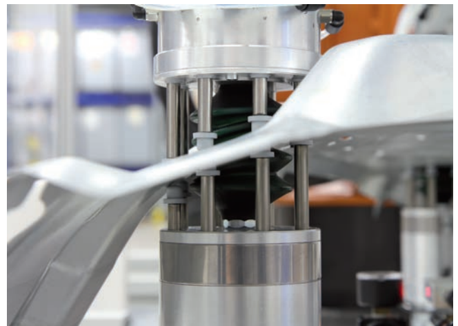
Suction Cup Balance SSCB clamping and handling a curved sheet for a car body
