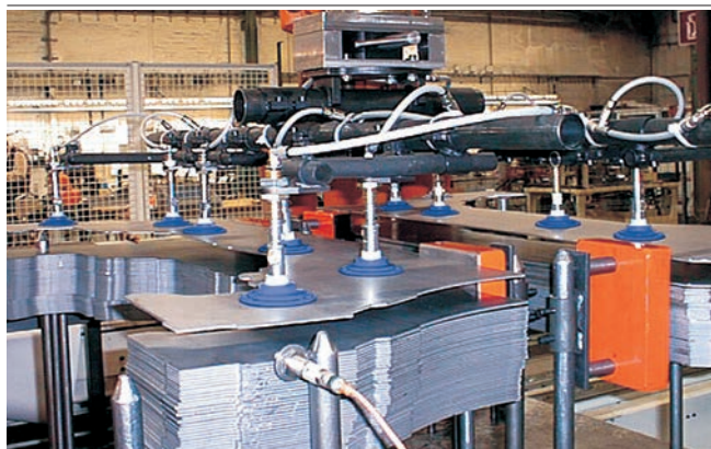
Mounting example Spring Plungers FSTE-HD
