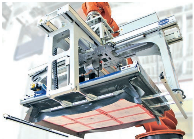
Layer gripping system SPZ with a suction area and global vacuum chamber palletizing beverage trays in layers
