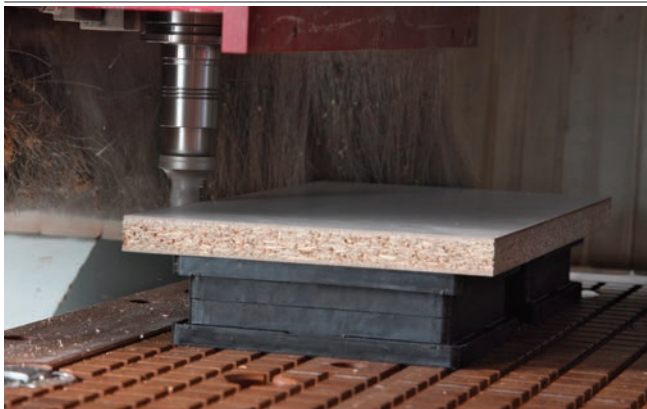
Vacuum block VCBL-R for gripping particle boards
