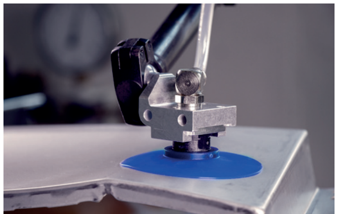
Holder for suction cup HT-SG with bell-shaped suction cup SAX for handling formed sheet metal parts
